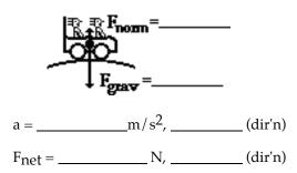
g. A 900-kg car makes a horizontal turn at 15.0 m/s around a curve with a 32.5-m radius of curvature.
