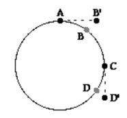
If the acceleration of the body is towards the center, what is the direction of the unbalanced force? Using a complete sentence, describe the direction of the net force that causes the body to travel in a circle at constant speed.
