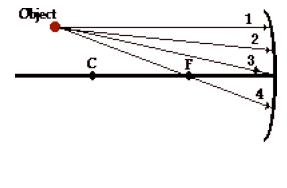
9. Consider the diagram at the right of an object, an image, and a concave mirror. On the diagram, show the path of light from object to the mirror to the eye as the eye sights at the image.
