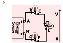
Given the circuit at the right with the listed current and resistance values, determine the electric potential at the indicated positions. Note that you are to find the electric potential (or voltage) and **NOT** the electric potential difference (or voltage drop).
