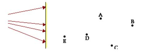
7. The diagram below depicts the path of four reflected rays that originated at the object on the left side of the mirror and have subsequently reflected from the mirror. Five lettered locations are shown on the right side of the mirror. Which location is representative of the image location?
