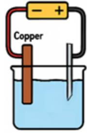
4. Sketch an electrolytic cell for the electrolysis of copper(II) sulfate using copper electrodes. Label:
