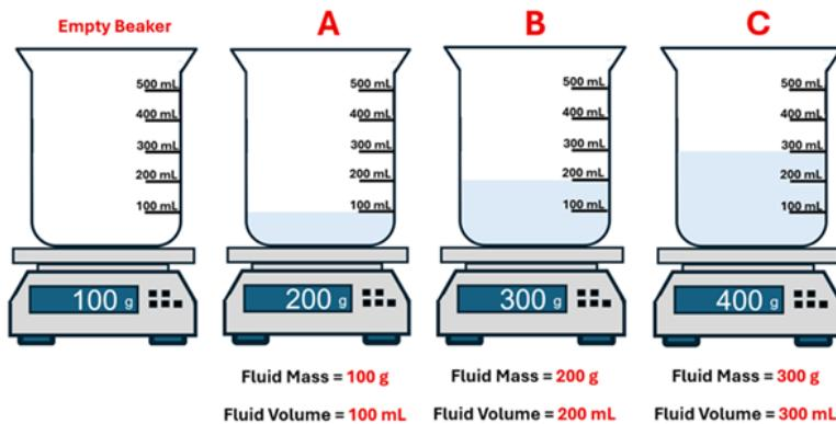
“4 beakers on top of scales are shown. Labels of Empty, A, B and C are above them, and the fluid mass and fluid volume are listed below. Empty shows 100g on the scale and no fluid in it (weight of the beaker), Flask A shows 200 g on the scale and a fluid mass of 100g and fluid volume of 100 milli liters. Flask B shows 300 g on the scale and has 200 g for mass and 200 milli liters of volume, and Flask C shows 400 g on the scale and has 300 g of mass and 300 milli liters of volume.”
