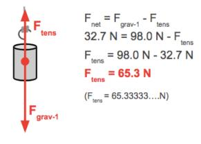
It doesn't matter which object is used for the Individual Object Analysis. The resulting calculation of tension will end up yielding the same value:
