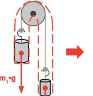
The system is commonly straightened out and pictured with competing gravity forces pulling in opposite directions.
