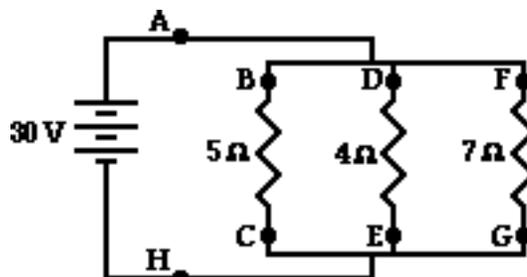
10. Determine the overall current in the circuit (as determined at position A or H).
