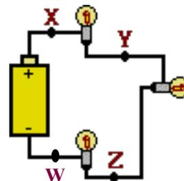
11. Three identical light bulbs are connected to a battery as shown below. W, X, Y and Z represent locations along the circuit. Which one of the following statements is true?
