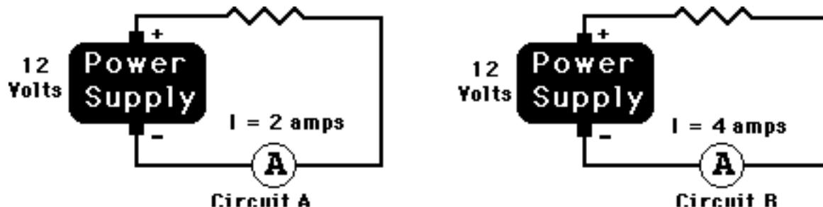
10. Use arrows to show the direction of conventional current flow through the following circuits and use the  $I = \Delta V / R$  equation to fill in the blanks.
