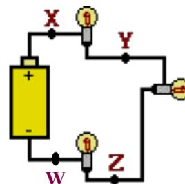
13. Compare a circuit with three light bulbs to a circuit with two light bulbs. All light bulbs are identical. In which circuit will the overall power be the greatest? Intelligently defend your answer.
